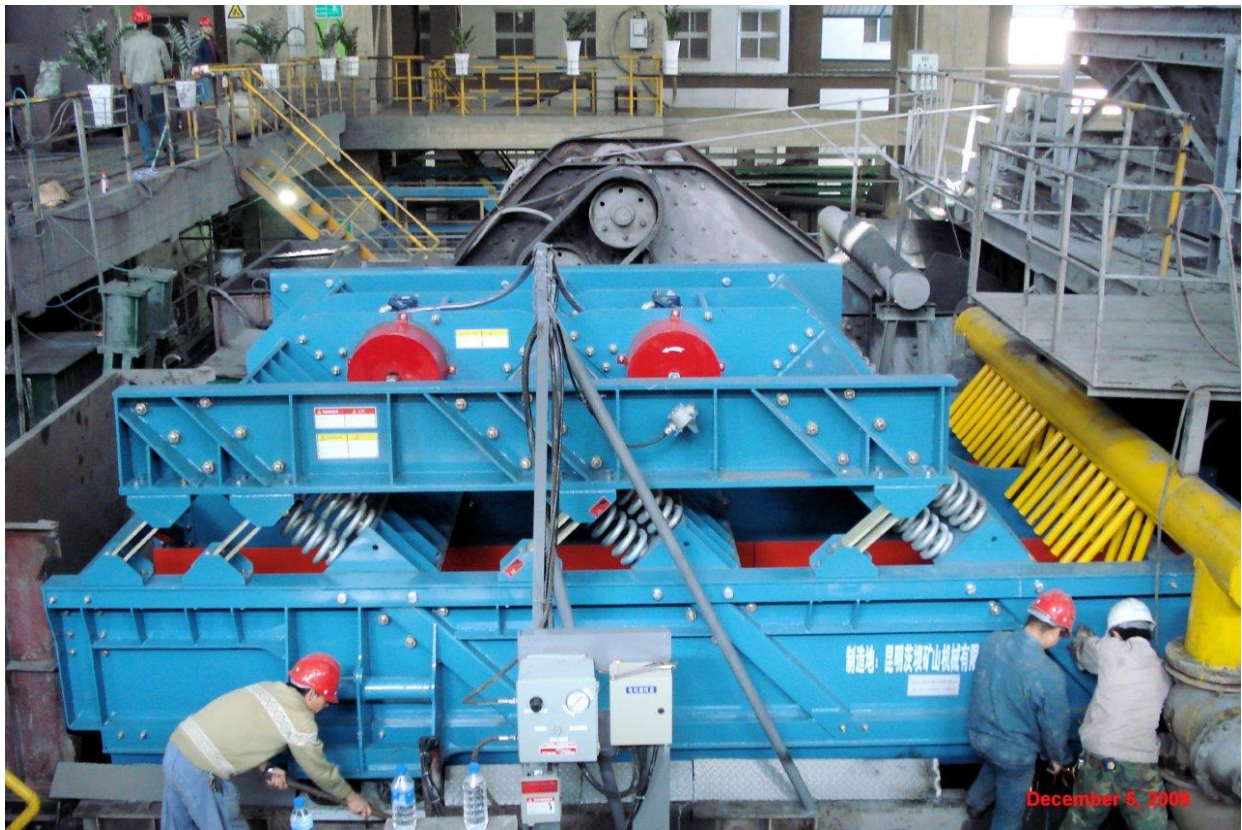
Fig 3 Dahongshan Iron Mine two mass Installation, old style behind (replaced 2010)
