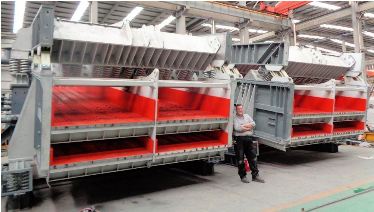
Fig 4 WA Iron Ore: 8 @ 3.6 m x 8.5 m two mass screens installed 2016, more ordered; Spec 3100 t/h, 2.24 sg, -22 / -12 mm cut, 90% / 85% passing; Operating at 4000 t/h
