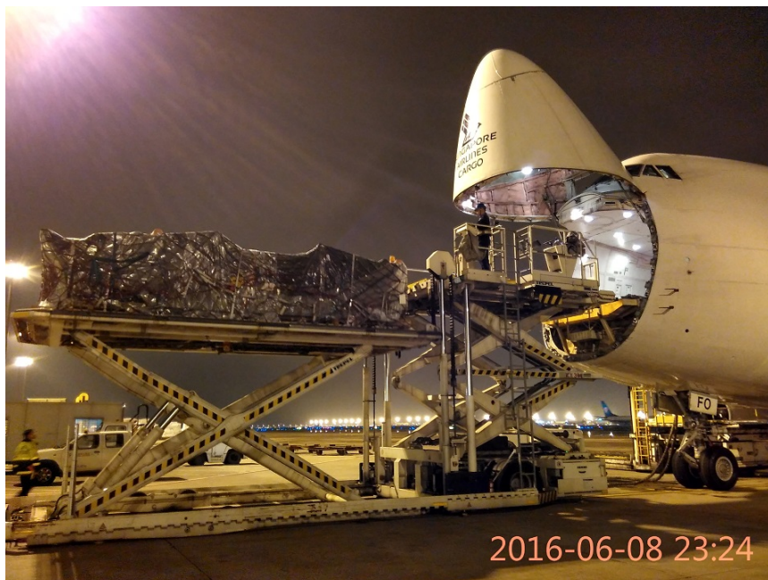
Fig 8 Half of a 3.6 m x 6.1 m two mass screen being loaded for air freight
