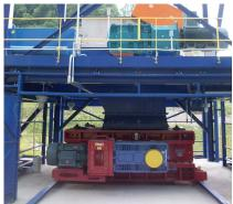
DDC-Sizers can be installed on rails for easy, safe access.
