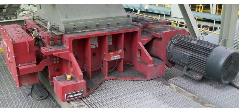
McLanahan DDC-Sizers provide primary, secondary and tertiary reduction of friable, low silica materials. They are frequently used in applications that include coal, salt, gypsum, phosphate, limestone, bauxite, petroleum coke, lignite, trona, oil sands, clay, shale and more.
