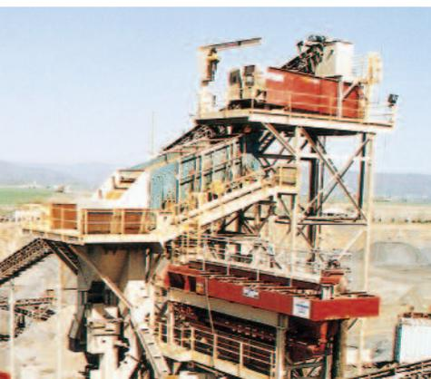
**McLanahan Aggregate Conditioners are tough and efficient.** They are designed to scour, abrade and break down water soluble silts and deleterious clays from coarse rock and/or sand and are placed ahead of wash screens to improve screening efficiencies or in front of a Sand Tank or Fine Material Screw Washers to improve the Sand Equivalency (SE).
