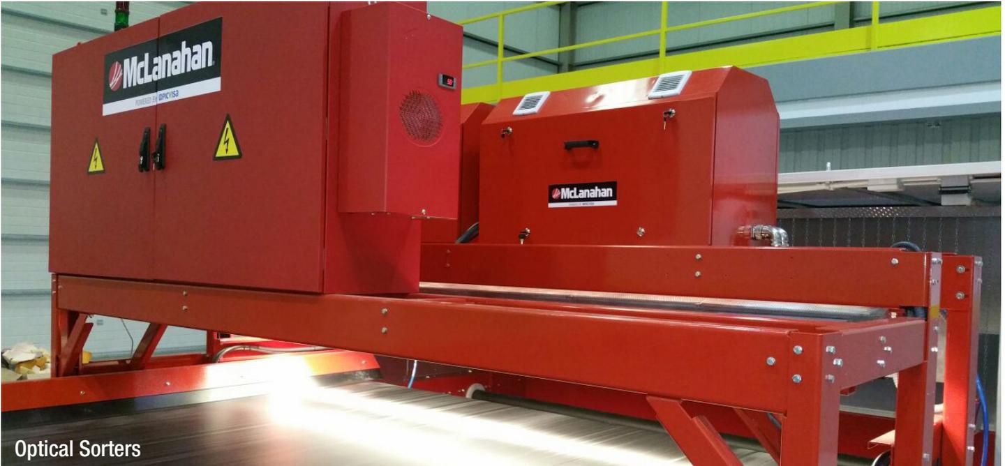
**Automated sorting involves using state of the art optical sorting technology, specifically utilizing NIR and/or Color technology to differentiate between different materials. Computers take the images from the camera to quickly and efficiently select which materials to positively or negatively sort.**
