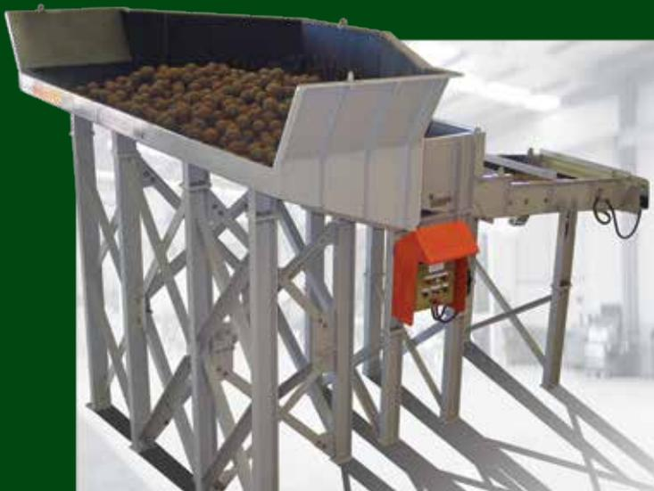
Tonnes of grinding media, normally in the form of steel balls, are consumed by all process plants having mills as part of their comminution process. The handling of heavy steel balls can be a safety issue when drums of balls are hoisted and tipped, often manually, into chutes and mill inlets.
