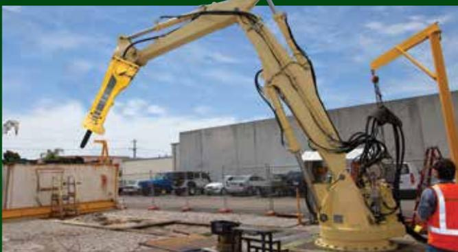
To ensure absolute reliability from first start-up, Transmin insists on complete trial assembly and test running of all our booms prior to commissioning. Transmin has a dedicated assembly and testing workshop which provides a clean environment for mechanical fitting and testing, as well as the ability to handle large quantities of booms efficiently and without delay. Client witnessing of testing is welcomed.
