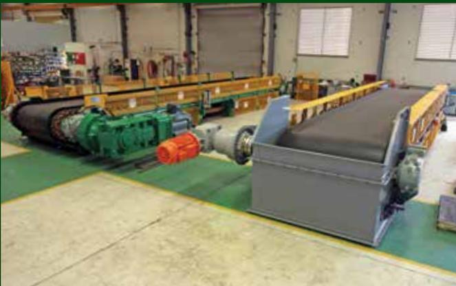
Since inception in 1987, Transmin has been designing and supplying bespoke belt feeders for mining and general industrial applications. In the early days these were mainly medium duty machines which sometimes incorporated load cells to accurately control or monitor material feed to process.
