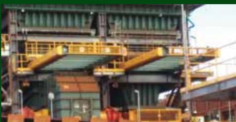
Ideal for screen house applications, safety isolation gates completely isolate feeders for maintenance.
