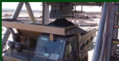
Clam gate for truck loading, of the single or double clam design, for loading control.
