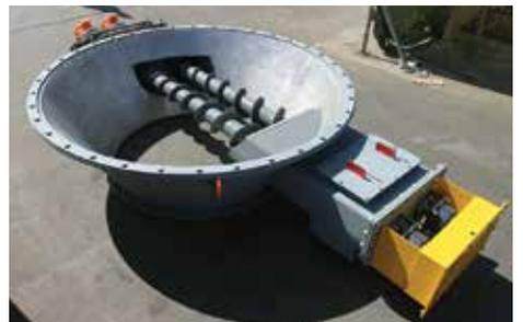
Special screws and feeders for difficult applications.
