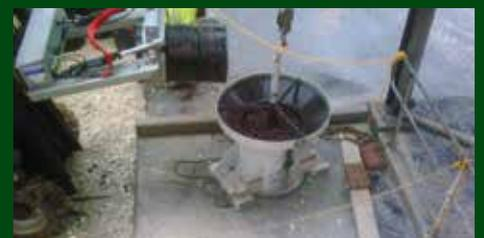
Hoist operated kibble option is the simplest solution for low ball consumption.
