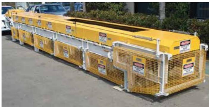
Special belt feeder for sample plant application.
